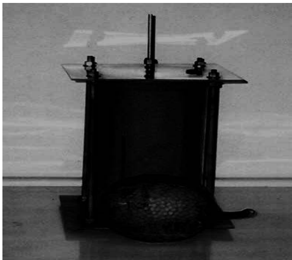
Figure 5. Breadfruit sample stored at Controlled Atmosphere with diffusion channel (CA).
